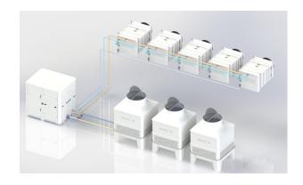
The other two core components of Dragons are the Regeneration Towers and the Conditioners. The Regeneration Towers are where the humidity extracted from the indoor environment is ejected from the closed circuit. The conditioners on the other hand is where the air brought into the closed liquid desiccant circuit in order to dehumidify, filtre and condition the air to supply it into the indoor environment.
